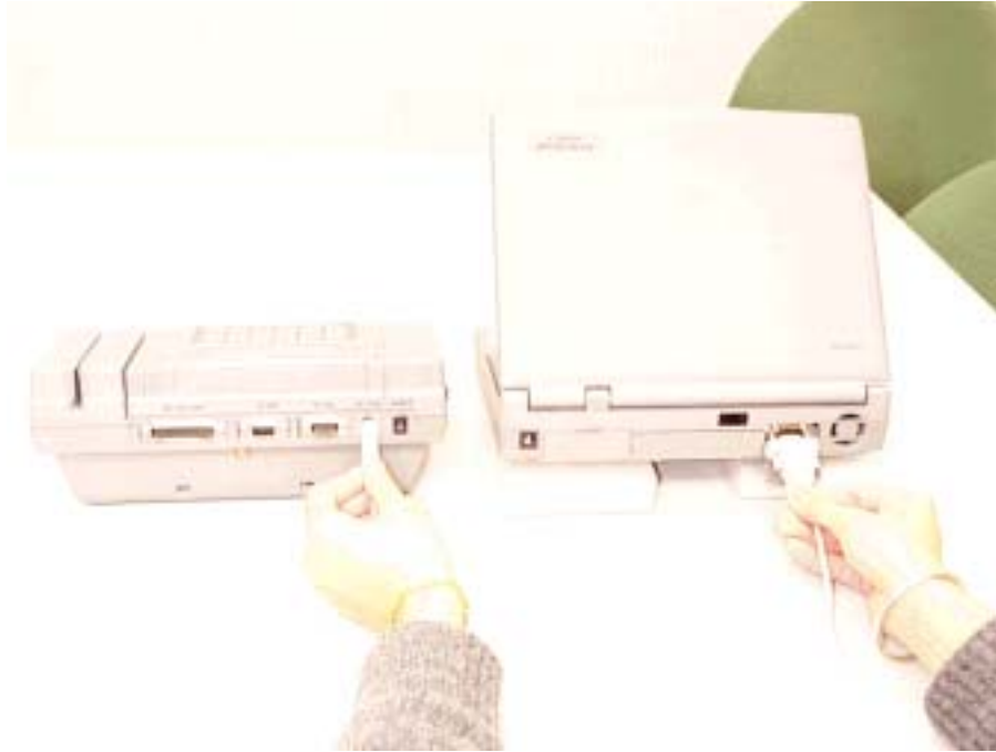
Figure 4-12 RS-232 Connection between Cipher-510 and Host
