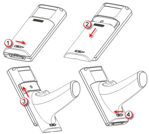
Figure 3: Installing the Pistol Grip
