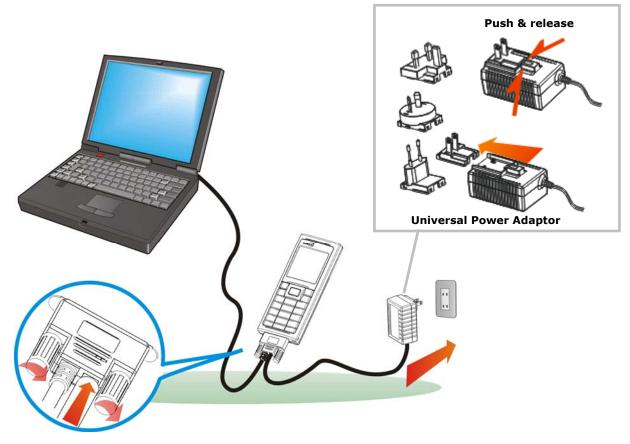
Figure 6: Using USB/RS-232 cable
