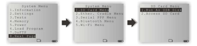
Note: When SD card is present, the card icon will appear flashing while being accessed. If the mobile computer is preloaded with Batch AG runtime, it will automatically create two working directories "\AG\IMPORT" and "\AG\EXPORT" on SD card.
