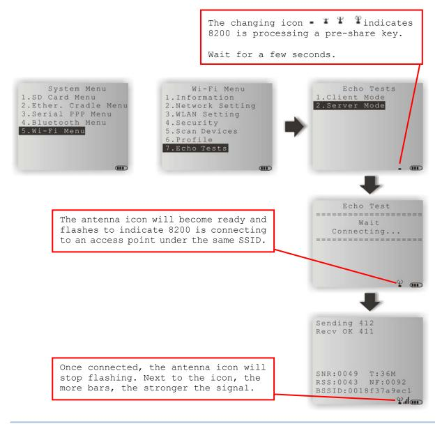
Note: If you are programming in C or BASIC, be aware that the antenna icon will appear on the device screen after NetInit() or START TCPIP() is called. (WPA must be enabled first!) Once the connection of echo test is established, the details will be displayed as illustrated below.
