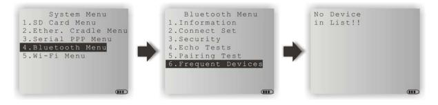
Note: To unpair any device, simply delete the device from this list.
