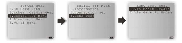
Note: To verify the connectivity of the Modem Cradle, run **System Menu | 3. Tests | 6.** Echo Test | 2. MODEM.
