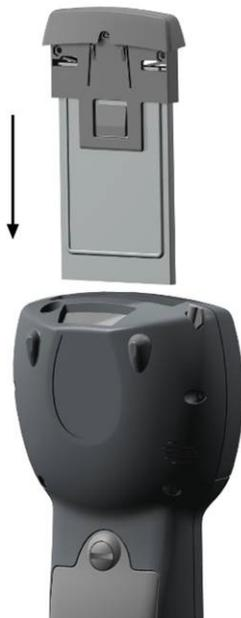
8. The card remains firmly attached to the antenna cover and is locked into place when inserted into the Nordic ID PL2000 unit.
