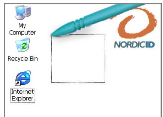
the corner of the selection box is above the pen tip, you will probably experience difficulty in selecting the taskbar at the bottom of the screen. If the selection box is a millimeter or two below the pens tip it does not require recalibration, it might actually aid a bit when accessing the taskbar. The sensitivity of the touch screen is also controllable, see the Touchscreen dialog in the Control Panel for the sensitivity setting.
