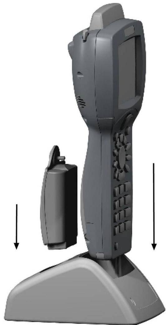
Figure 8: The Nordic ID2000 unit with the Desktop Charger.
