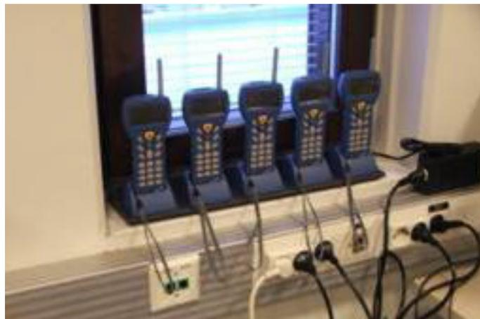
Picture: Write down the serial numbers of the handsets, install batteries in the handsets and, if necessary, change the settings according to the requirements of the installation location. The settings menu can be protected with a password. Finally place the handsets in the charger, so that you can check the charging function and charge the handsets fully for any possible training.
