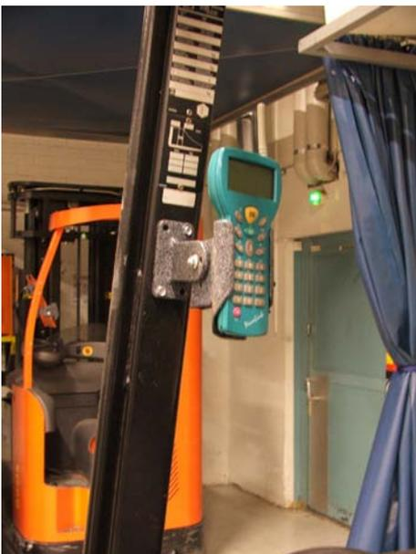
Picture: The stand for the RF600 and terminal, installed by forklift.
