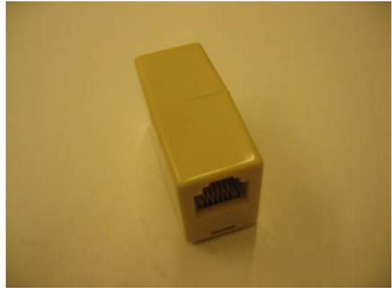
Picture: The extension cable set for the RF600 base station includes a connector for extensions (picture on the left) as well as a separate piece equipped with a voltage source connector, which is installed on the workstation end of the cable (picture on the right).
