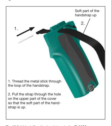
Pull the handstrap until the metal stick sets up to its holes.
