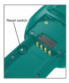
Fig.30 Reset switch of PL3000
