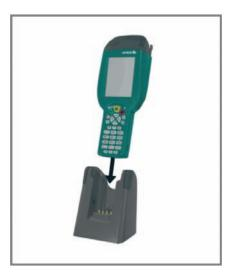
Fig.15 Placing the PL3000 to the charger
