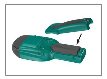
Fig.9 Remove the back cover
