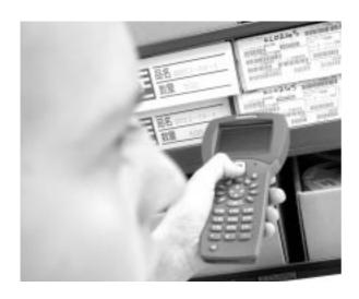
The built-in barcode scanner can be activated simply by pressing a button. The scanned data can either be stored in the local memory or transferred immediately to the company data system.
