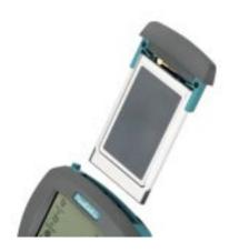
PiccoLink® 2000 can be used stand alone but it also connects to the company's wireless data network. PiccoLink® 2000 features a user-accessible full-size PC card type II slot accommodating, for instance, a GSM, WLAN or a GPRS card. For future the PiccoLink 2000 supports any technology that is provided in PC card format, eg. Bluetooth and GPS.
