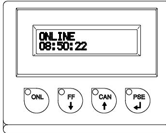
The control panel display constantly provides the operator with the actual information concerning the current printer mode and label processing. The indicator LEDs support the information shown in the display by indicating which keys have to be pressed. (e.g. in the event of a fault)
