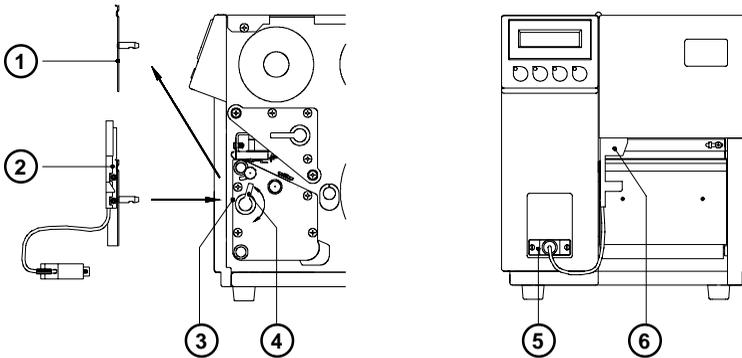
The **Apollo** is generally shipped with the tear-off plate (1) mounted. When operating in dispense mode, the tear-off plate has to be replaced with the present sensor (2) :
