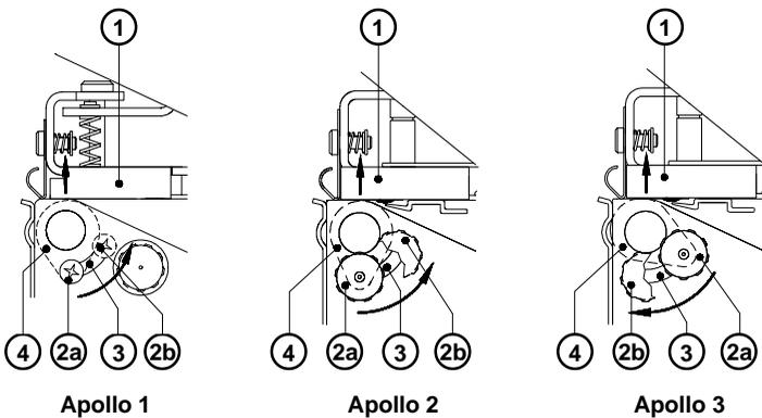
When printing narrow labels (width less than 2.5 in or 60 mm), it is possible that the printhead will come into direct contact with the drive roller. This will lead to premature wear on the printhead. In addition, the printhead will be at a slight angle to the label, thus, the uneven pressure may result in an inconsistent image density from one edge of the label to the other.
