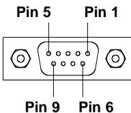
Pin 1/2 - Optocoupler inputs. A short impuls of 24V= at the pins (+ at pin 1, - at pin 2) releases the print of one label (external start signal). The start impuls has to be shorter than the print time of the label. The current is internally limited to 10 mA.
