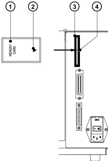
The front side of the memory card (1) is usually marked by the inscription "MEMORY CARD", and an arrow (2) representing the direction of inserting the card into the drive. There is also an arrow (4) impressed into the frame of the memory card slot of the **Apollo**.
