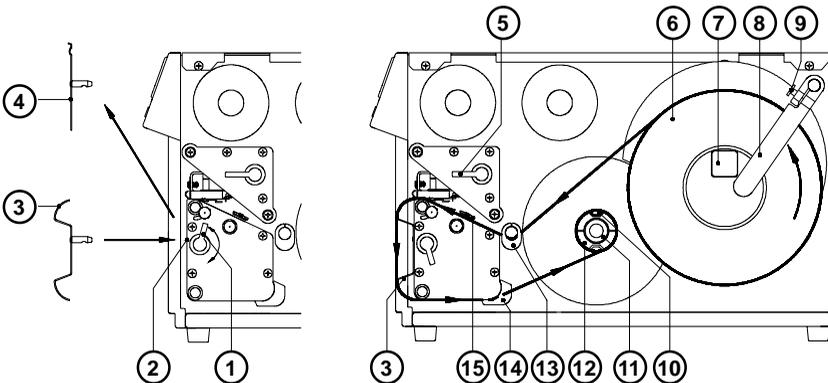
5. Lift printhead by turning the lever (5) clockwise until it stops.
