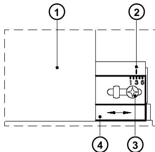
If creases, lines or black patches appear in the print image resulting in a poor print quality, this may be caused by wrinkles in the transfer ribbon (1). To remove the wrinkles, the tension of the ribbon should be made even from the left to the right by moving the ribbon shield (4) up or down.
