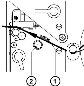
To accommodate a variety of print jobs, the position of the label edge sensor (1) can be adjusted at right angles to the path of the paper feed.
