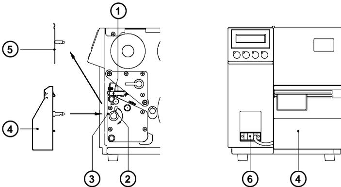
The **Apollo** is delivered with the tear-off plate (5) installed.
