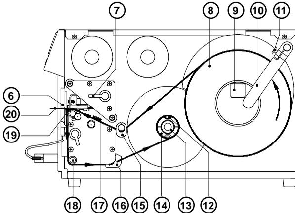
1. Lift the printhead by turning the lever (7) clockwise until it stops.
