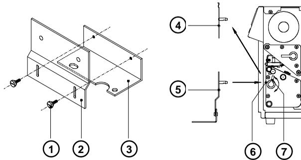
1. Attach upper adapter plate (2) to the lower adapter plate (3) using the knurled screws (1). Put the screws through the circular holes in the upper adapter plate.
