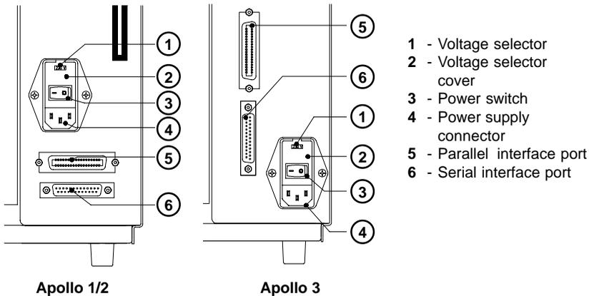
To change the voltage setting, open the cover (2) and remove the voltage selector from the power unit.
