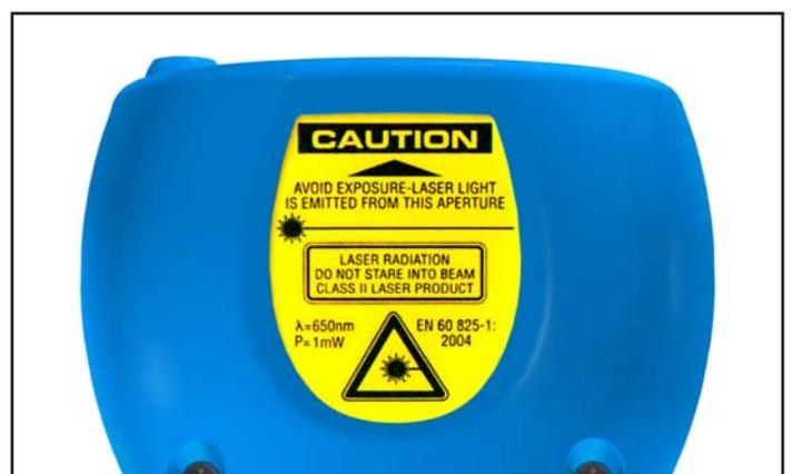
Fig. Laser safety label at backside of the RF651
