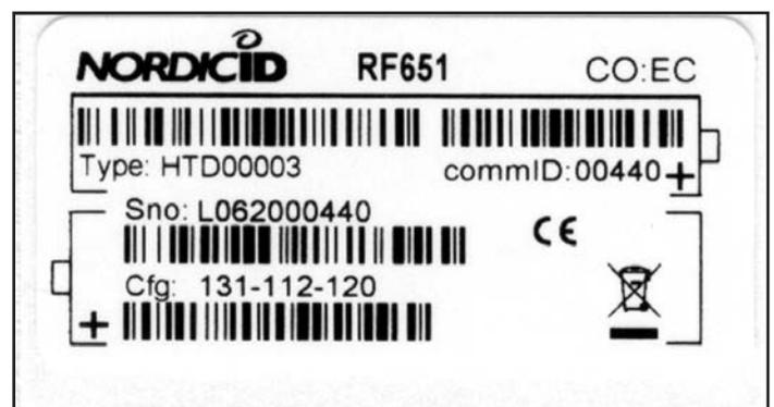
**Fig.** Type plate of the RF651.
